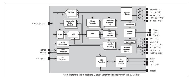
The BCM5478 consists of eight complete 10/100/1000BASE-T Gigabit Ethernet transceivers integrated on a single monolithic CMOS chip. The BCM5478 is optimized for low power and small footprint size to enable high-port-density applications. The BCM5478 enables a new class of cost-effective Gigabit Ethernet equipment by lowering system cost and reducing power dissipation by nearly 30 percent, driving the delivery of Gigabit Ethernet bandwidth to the desktop.
